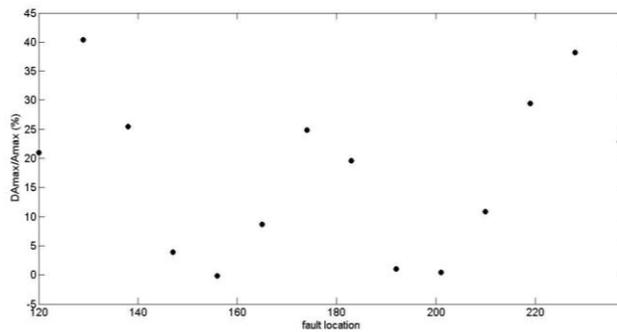
Figure 13- Dependency of maximum points of input impedance to fault location in the second layer
