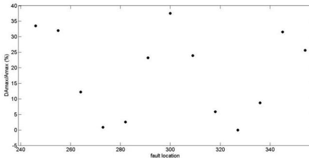
Figure 14- Dependency of maximum points of input impedance to fault location in the third layer
