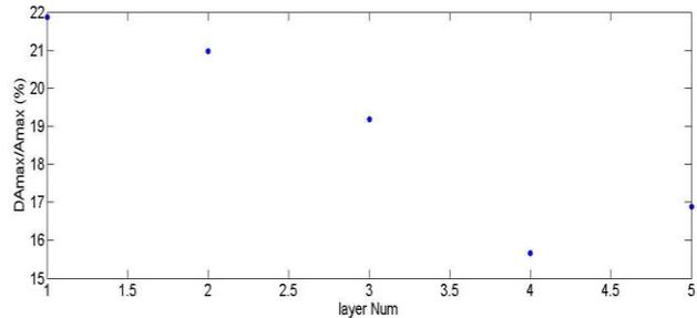
**Figure 21-** Dependency of maximum points of input impedance according to layer number
