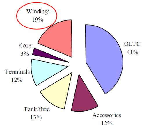
Figure 1- Different fault percentage in transformer [3]
