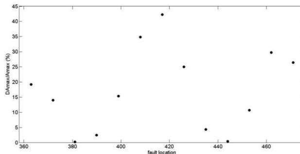
Figure 15- Dependency of maximum points of input impedance to fault location in the fourth layer
