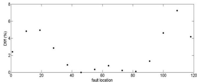
Figure 12- Frequency dependence of maximum points of input impedance to fault location in the first layer
