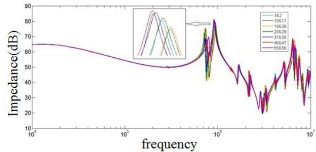
**Figure 8-** Frequency response of winding with the existence of various faults in the first layer
