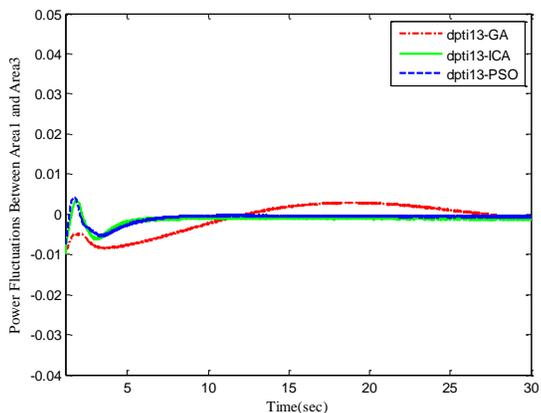
Fig. 15 Power fluctuations between area1 and area3 by using PID controller
