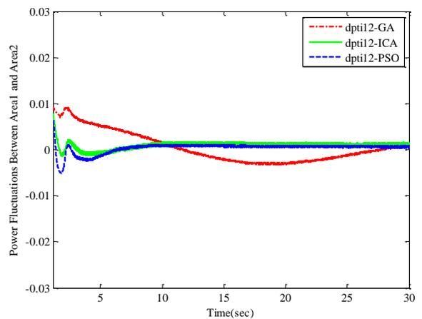
Fig. 14 Power fluctuations between area1 and area2 by using PID controller
