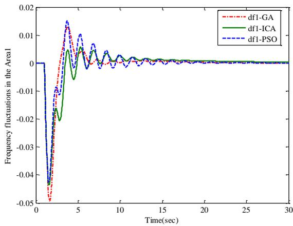
Fig. 11 Frequency fluctuations in the area1 by using PID controller
