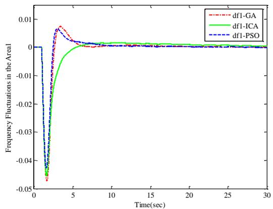
Fig. 17 Frequency fluctuations in the area1 by using PSS-AVR
