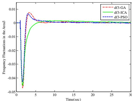
Fig. 19 Frequency fluctuations in the area3 by using PSS-AVR
