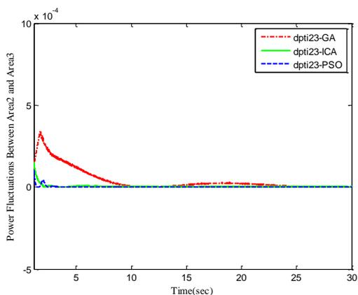
Fig. 16 Power fluctuations between area2 and area3 by using PID controller
