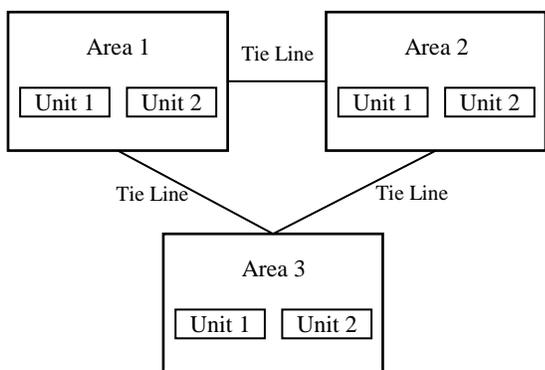
Fig. 1 Three-area generalized AGC block diagram.
