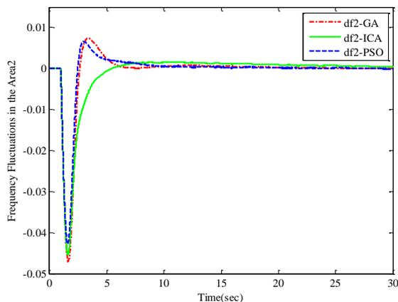
Fig. 18 Frequency fluctuations in the area2 by using PSS-AVR
