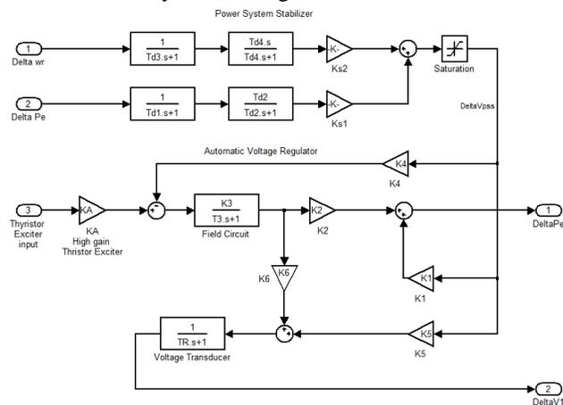
Fig. 6 AVR system controlled by PSS
