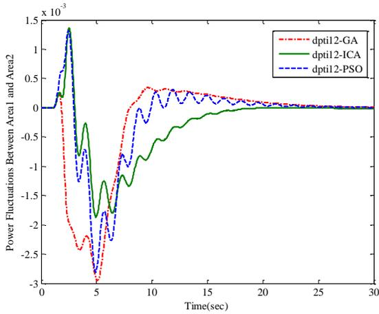
Fig. 20 Power fluctuations between area1 and area2 by using PSS-AVR
